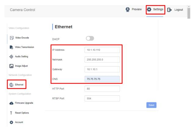
Change the camera's default IP and DNS so that they're consistent with router's settings. For IP address, make sure the first 3 sections are the same as IP1. On Page 1 of this instruction, we noted IP1 is 10.1.10.151, thus here we change the "IP Address" (IP3) to 10.1.10.110. Netmask: 255.255.255.0, Gateway: 10.1.10.1, DNS: 75.75.75.75. Click "Save" to save the settings.
