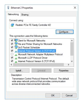
Choose "Use the following IP address", change computer "IP address" (referred to as IP2) to be consistent with the camera IP address (referred to as IP3). For example, AV-2020 default IP address (IP3): 192.168.1.188, thus the user can change the computer IP address (IP2) to 192.168.1.100. Make sure the first 3 sections are the same. Subnet mask: 255.255.255.0, default gateway: 192.168.1.1. Click on "OK". In the warning window, click on "Yes".
