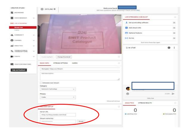
At the bottom of "Stream now" page (red circle), there's the "ENCODER SETUP" section, in which it contains "Server URL" ad "Stream name/key". Click "Reveal" so you can see the "Stream name/key" for a few seconds.
