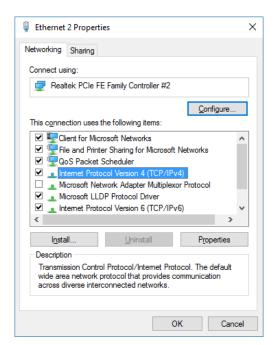
Choose "Use the following IP address", change computer "IP address" (referred to as IP2) to be consistent with the camera IP address (referred to as IP3). For example, AV-1361 default IP address (IP3): 192.168.5.163, thus the user can change the computer IP address (IP2) to 192.168.5.100. Make sure the first 3 sections are the same. Click on "OK". In the warning window, click on "Yes".
