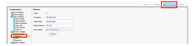
Find the "IP Address" and change it to be consistent with IP1 (router IP). Make sure the first 3 sections are the same. For example, at the beginning of this instruction, notice IP1 is <u>10.1.10.</u>151, then the user can change the "IP Address" (IP3) to <u>10.1.10.</u>110. Click on "Save" to save the change.
