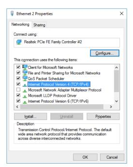
Choose "Use the following IP address", change computer "IP address" (referred to as IP2) to be consistent with the camera IP address (referred to as IP3). For example, AV-1361 default IP address (IP3): 192.168.5.163, thus the user can change the computer IP address (IP2) to 192.168.5.100. Make sure the first 3 sections are the same. Click on "OK". In the warning window, click on "Yes".
