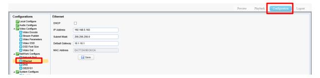
Find the "IP Address", and change it to be consistent with IP1 (router IP). Make sure the first 3 sections are the same. For example, at the beginning of this instruction, notice IP1 is <u>10.1.10.</u>151, then the user can change the "IP Address" (IP3) to <u>10.1.10.</u>110. Click on "Save" to save the change.
