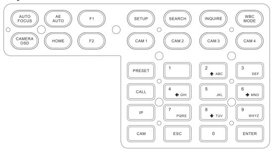
【AUTO FOCUS】 Set the camera to auto focus mode with this button. It will light up when camera is in manual focus mode.
