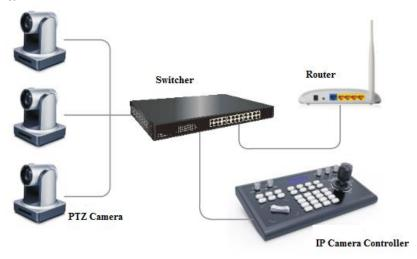
The controller and PTZ camera must be connected within the same LAN. IP addresses need to be set at the same segment.
